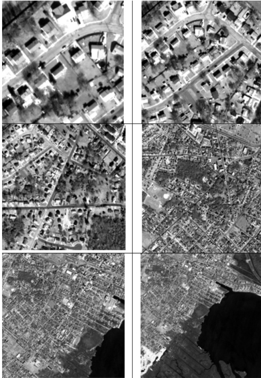
Figure 10. QuickBird sub images showing 0.6 m, 1 m, 2 m, 5 m, 10 m and 15 m ground resolution (from Jacobsen 2005)
